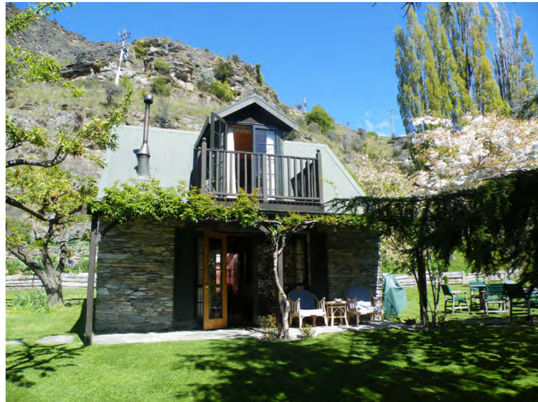
Trelawns Cottage (Arthurs Point) – using the roof void to create a habitable room within a constrained building envelope
