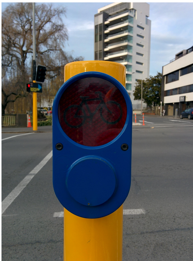
Figure M01 – Cycle call accept indicator (no call present).
