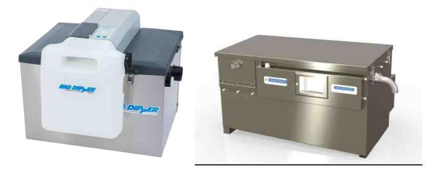
This type of equipment, often referred to as <u>G</u>rease <u>R</u>emoval <u>U</u>nits (GRU's), operates by trapping larger solids in a basket then removing the float layer of FOG from the unit by means of a slotted skimming wheel or electrostatic drum which is directed to an external container. The FOG may then be recycled or disposed of as 'solid' waste. Sediment once again settles at the bottom of the unit.
