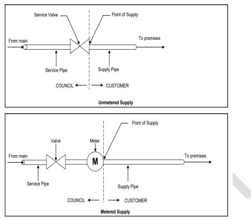
Figure 1 Typical Layouts at point of supply
