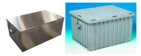
This type of equipment consists of a 'box' in which wastewater is temporarily 'held' while a pre-treatment medium (bacterial or enzyme based: see comment later in this section regarding the action and usage of these media) acts on the float layer of FOG. Sediment, as the term suggests, falls to the bottom of the 'box' forming a layer.
