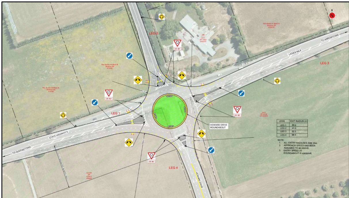
Figure 18: Proposed roundabout on the intersection of SH6 and Howards Drive (note that the final positioning at this location is to be confirmed)
