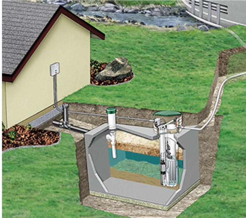
Figure 2: A typical on-property septic tank pump system. In both instances, wastewater is pumped from the property to a treatment plant via a public reticulation system.
