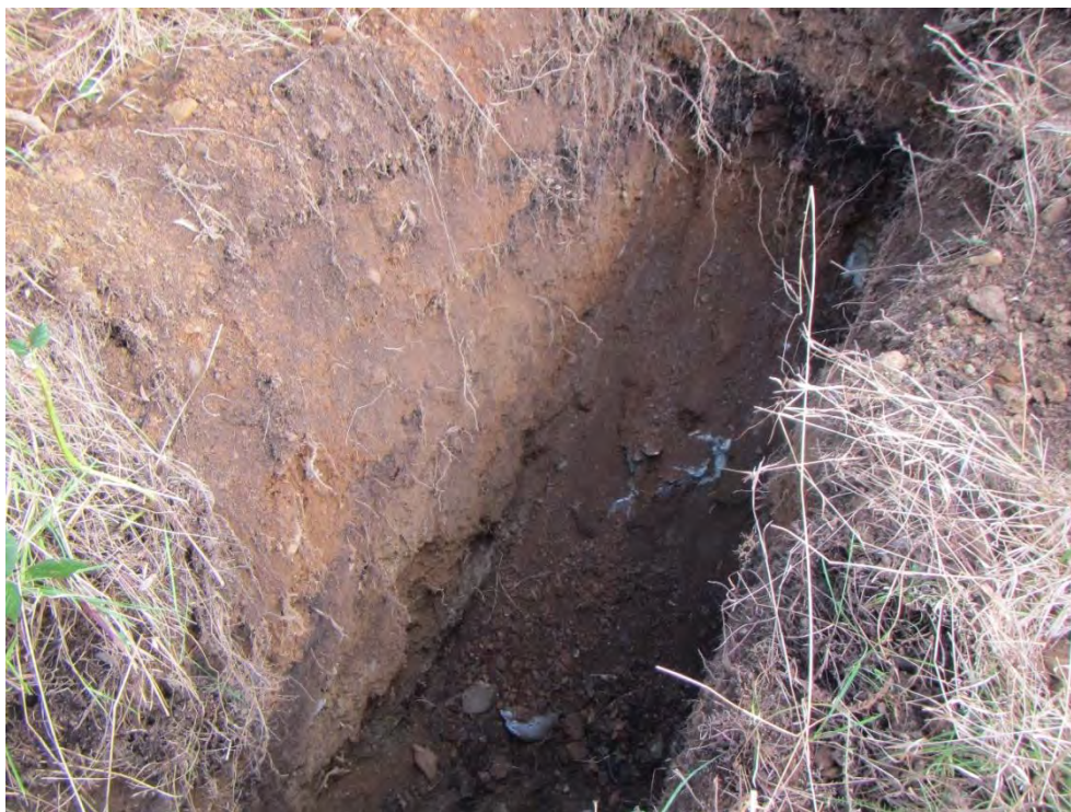
Plate 1: Soil test pit in the upper western part of the site, showing deep soil with schist bedrock in the base of the pit.
