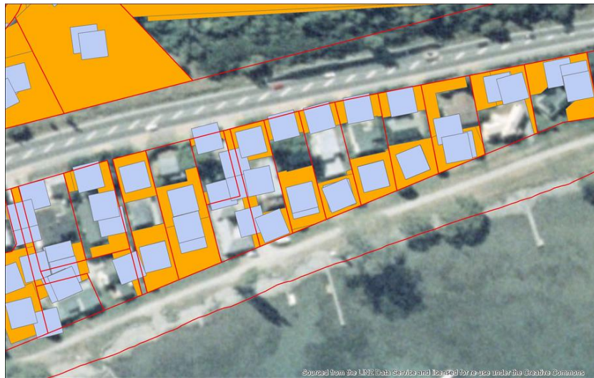
Figure 6 - Testing for Minimum Site Shape Requirement
