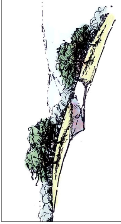
SKETCH 5 - NOT THIS Driveway Grading too Abrupt
