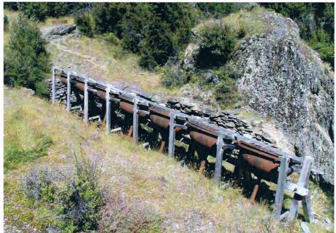
The seven berdans still located at Invincible Mine site, photo courtesy of Department of Conservation
