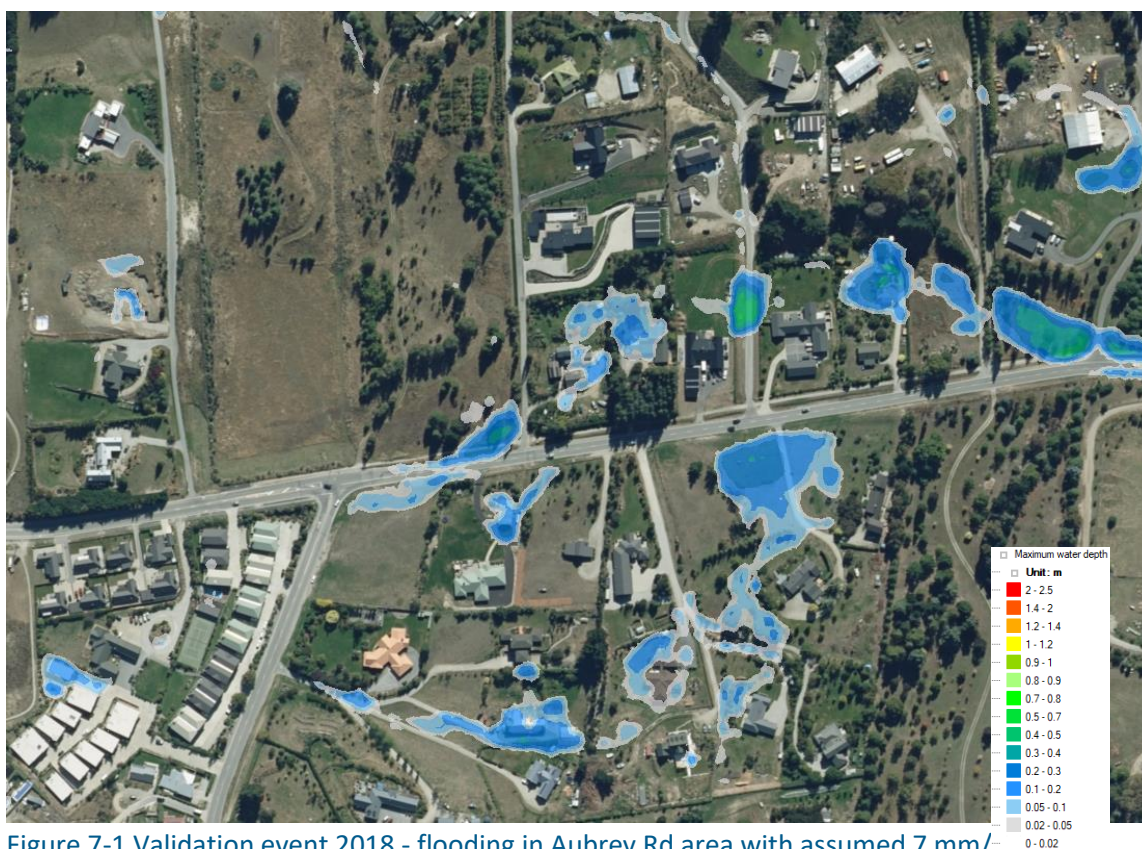
Figure 7-1 Validation event 2018 - flooding in Aubrey Rd area with assumed 7 mm/hr infiltration for pervious areas and soakpits infiltration of 200 mm/hr
