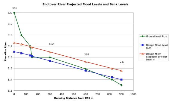
Figure 3.5: Recommended stopbank OR hardfill levels compared with existing ground level on left bank
