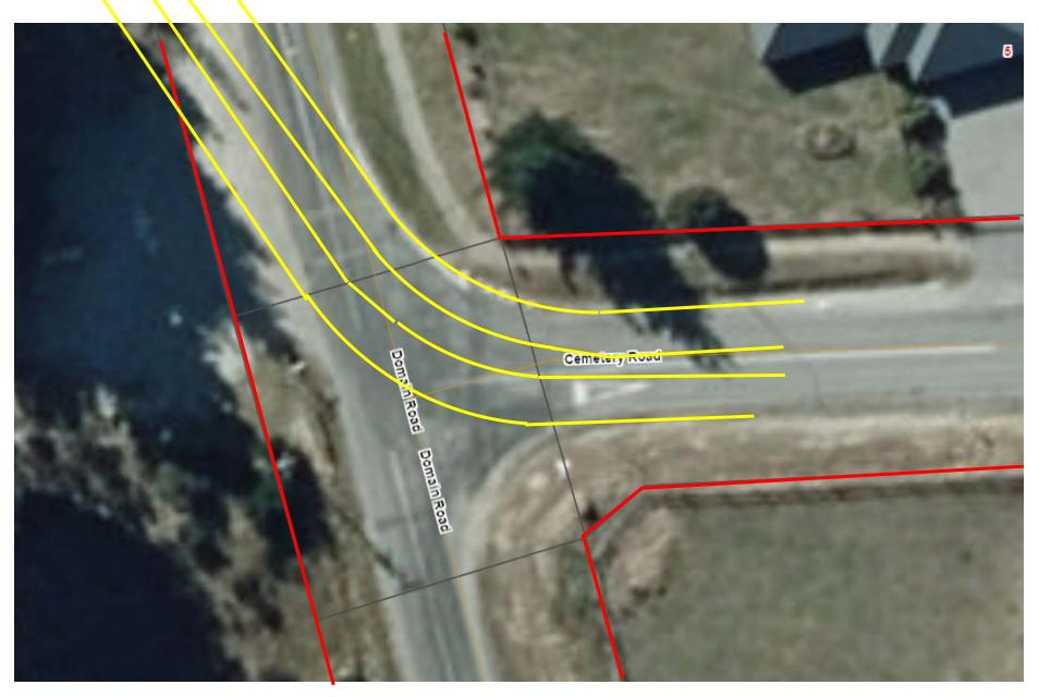
Figure 4: Domain Road / Cemetery Road Intersection, with Frankton Road / Stanley Street Intersection Main Carriageway Markings Overlaid
