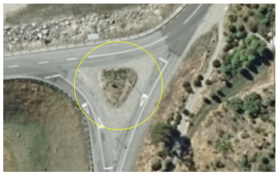
Figure 1: 30m Diameter Circle Overlaid at Domain Road / Capell Avenue Intersection
