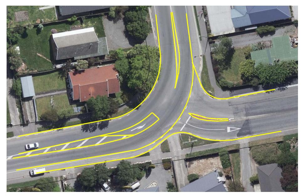
Figure 8: Ivory Street / Northbrook Road Intersection, Rangiora with Carriageway Markings Traced in Yellow
