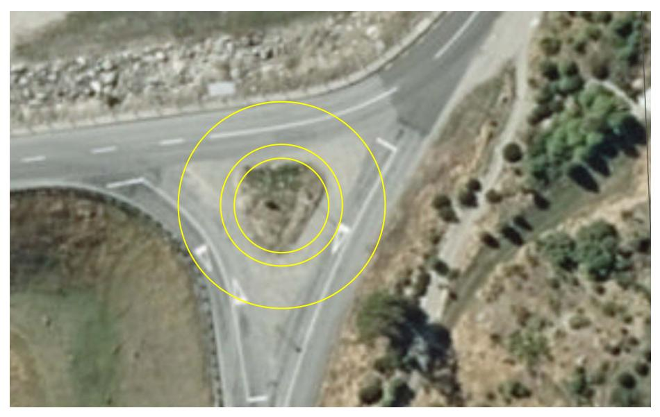
Figure 4: Central Island and Outer Diameter of State Highway 84 / Anderson Heights Roundabout Overlaid at Domain Road / Capell Avenue Intersection
