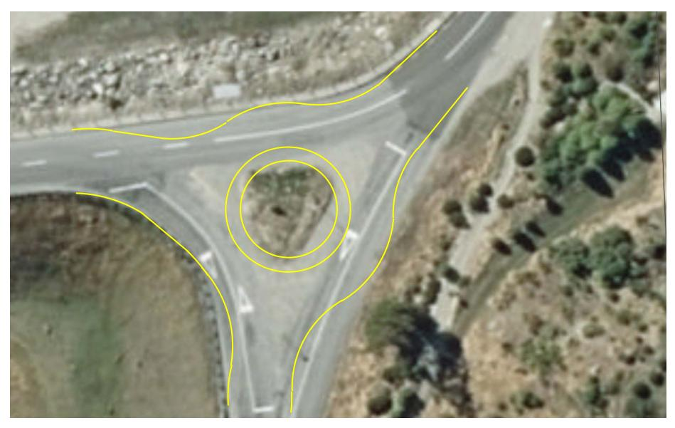
Figure 5: Possible Domain Road / Capell Avenue Roundabout Based on Geometry of State Highway 84 / Anderson Heights Roundabout
