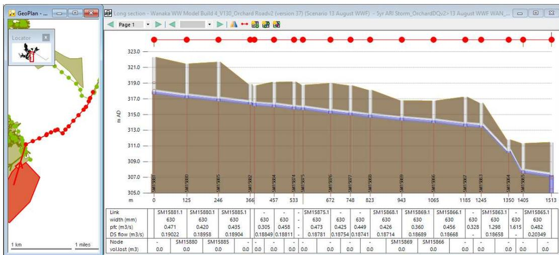
FIGURE 4-2 ORCHARD/RIVERBANK ROAD (26 L/S FLOWS) TO TRANSMISSION – 5 YEAR ARI DESIGN STORM
