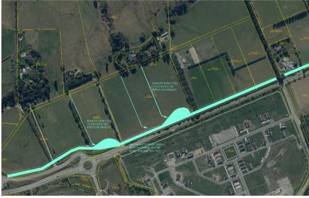
Figure 5 – Swales versus piped networks and impact on basin sizing
