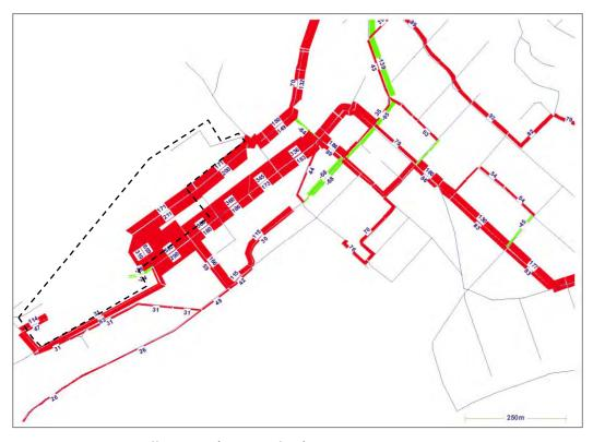
Figure 11: Change in traffic volume (two-hour flow) due to Plan Change, PM Peak, 2026
