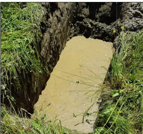
Photo 3: Indicates groundwater 800 mm below surface of Test Pit 8
