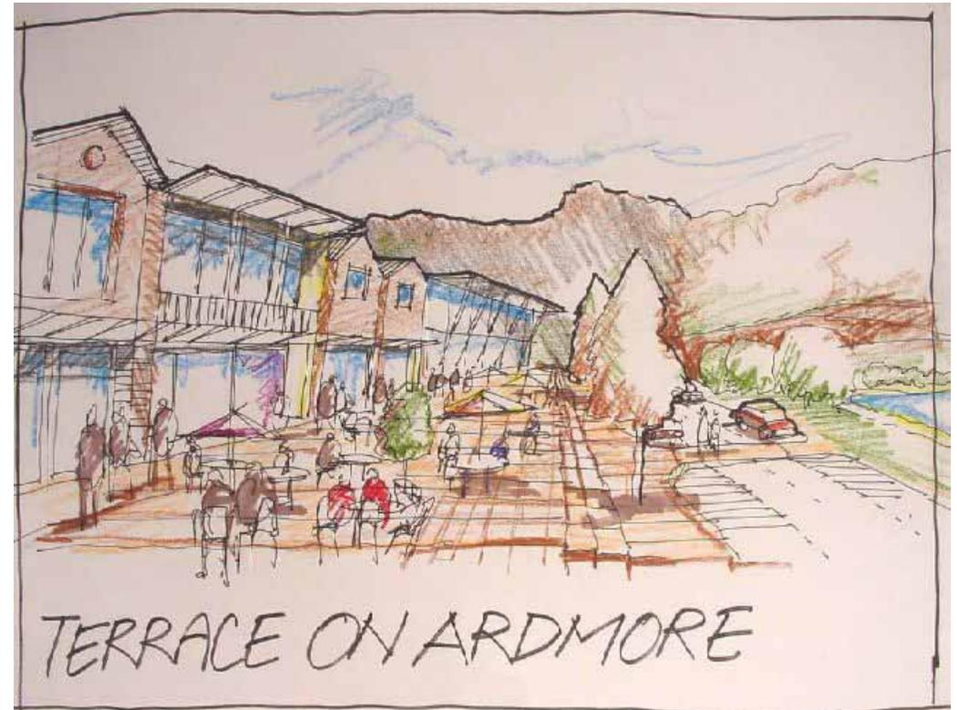
Drawing 4 – Comprehensive new development build with ground floor levels above flood level and with a broad, split level pedestrian promenade and all ground level premises accessed from the upper level of the promenade.
