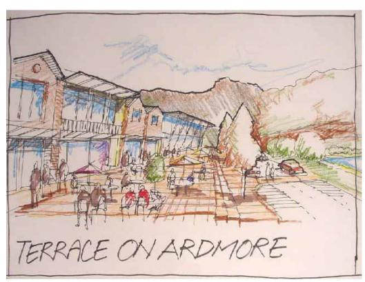
Drawing 4 – Comprehensive new development build with ground floor levels above flood level and with a broad, split level pedestrian promenade and all ground level premises accessed from the upper level of the promenade.
