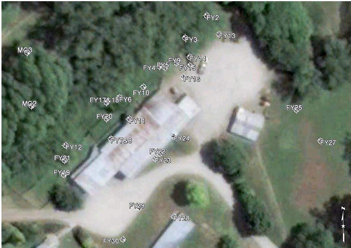
Figure 33: Closer view of sampling locations around the Barn/woolshed & Yards environs showing the sampling pattern in the inferred/most likely location of the former sheep dip. Sample locations in the figure are marked with a white circle with quadrants and sample names appear in white alongside quadrant markers (Google Earth Image).
