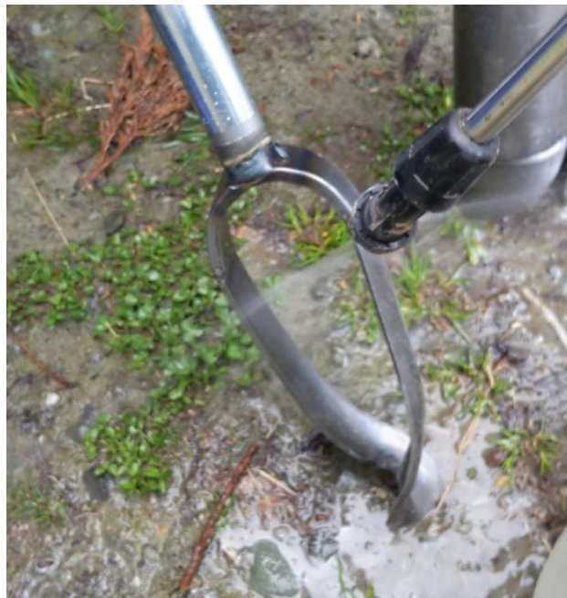
Figure 34: The sampling auger being washed with a pressure sprayer.
