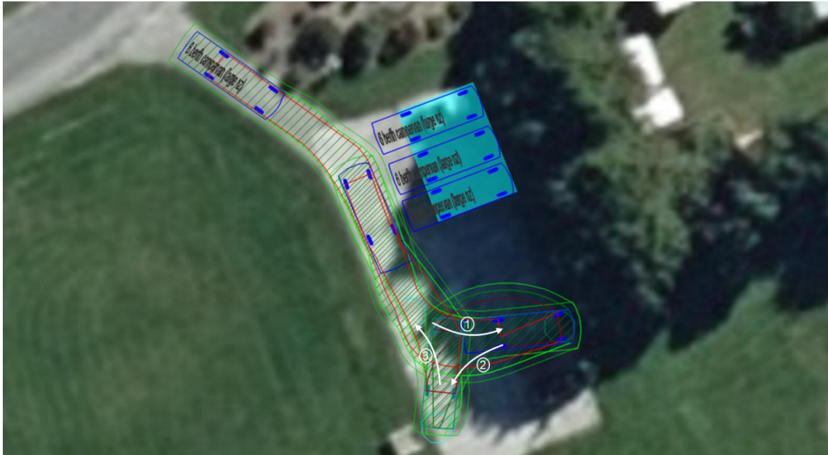
Figure 3.1: Glenorchy Domain Carpark Campervan manoeuvre to enter and exit the site if the freedom camping spaces (in blue) are all occupied.
