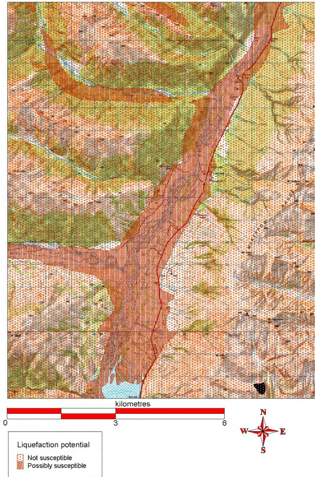
Figure 8: Land possibly susceptible to liquefaction induced by seismic shaking.
