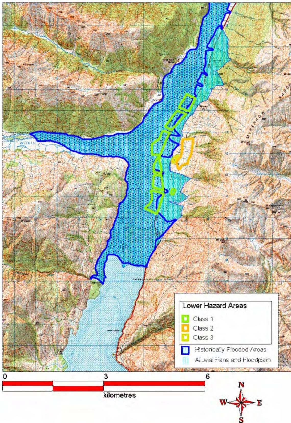
Figure 6: Combined flood and alluvial fan hazards, with lower hazard areas, Makarora valley.
