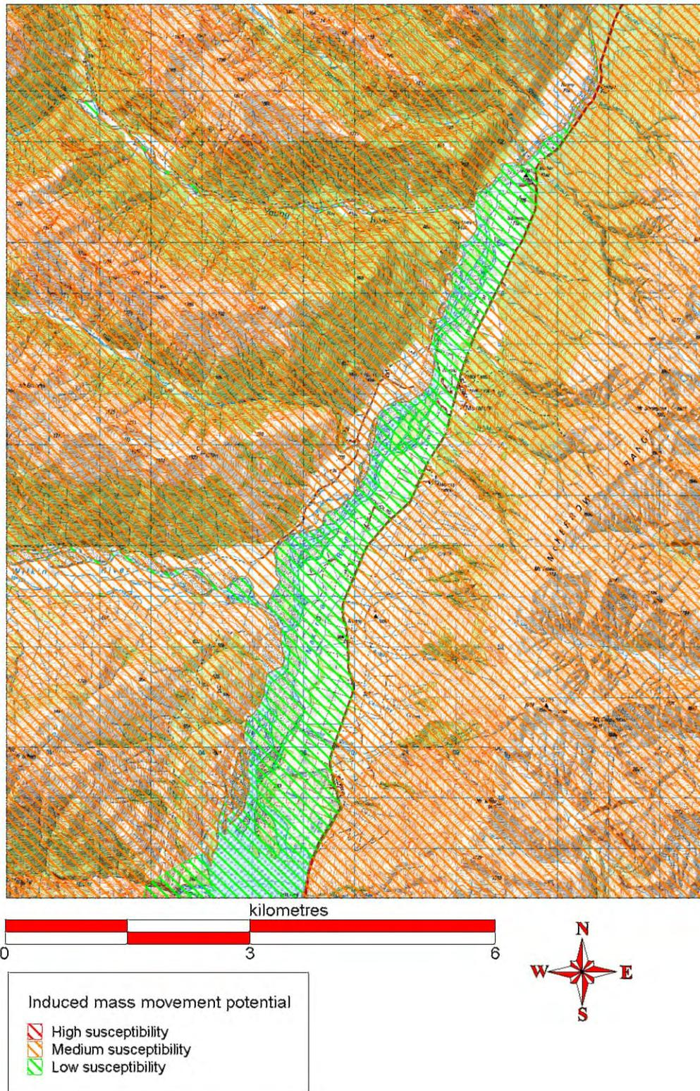
Figure 9: Susceptibility of land to mass movement induced by seismic shaking.
