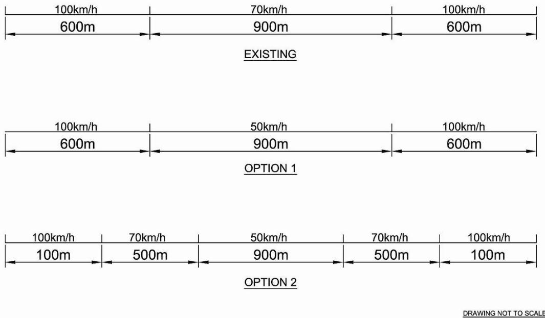
Figure 5 : Speed limit options tested
