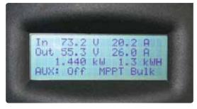
Example of a display unit on a grid-connected photovoltaic system.
