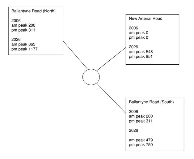
Figure 4 - Existing and projected morning and afternoon peak (2 - way) 2 hourly flow levels at the new arterial road intersection with Ballantyne Road.
