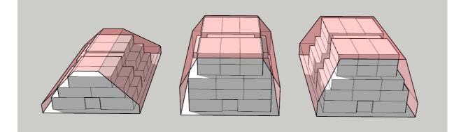
Figure 11 - Potential building envelopes for building height and sunlight admission controls for existing HDRZ (left), recommended option (middle), and alternative option (right).
