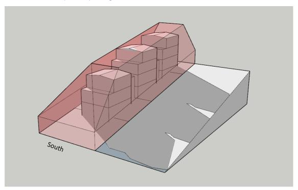
Figure 5 - Application of a 35<sup>o</sup> recession plane on the rear boundary a sloping site with an increased height limit to 11m. Model shot is taken at 3pm on 21 September with the models shown fully compliant with all standards.
