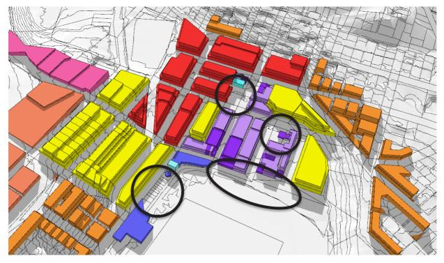
Figure 15 – Theoretical worst case (full development) sunlight access to town centre open spaces example. Model date of 21 July @ 10.30am demonstrates that the four main open spaces (Village Green, Earnslaw Park, St Peters Church and Marine Parade) within the town centre would still receive direct sunlight at certain times during winter months with recommended height increases. Note: adjacent HDRZ and PC50 areas have been shown for context.
