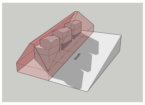
Figure 6 - Application of a 35<sup>o</sup> recession plane on the side boundary of a sloping site with an increased height limit to 11m. Model shot is taken at 3pm on 21 September with the models shown fully compliant with all standards.
