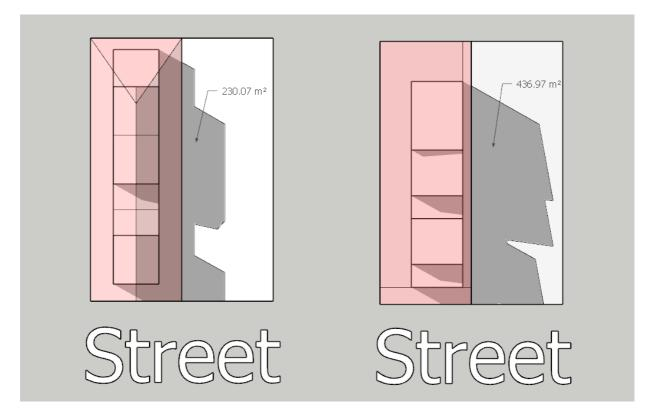
Figure 3 - Example difference in shading effects between flat (left) and sloping (right) sites under the PDP. Model shot is taken at 3pm on 21 September with the models shown fully compliant with all standards.
