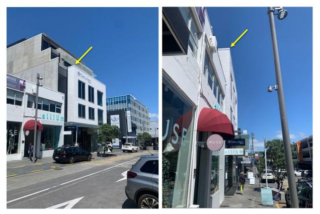
Figure 13 - Example of the application of upper-floor setbacks making upper-floors of a commercial building "disappear" at street level
