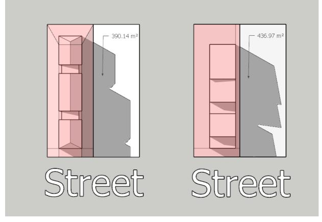
Figure 4 - Option 1 amendments on the flat site (left) vs existing standards on a sloping site (right). Model shot is taken at 3pm on 21 September with the models shown fully compliant with all standards.
