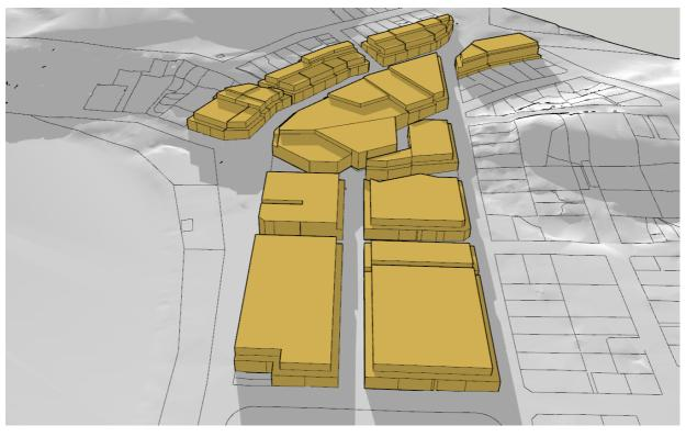
Figure 16 - Wānaka Bulk and Scale (at 20m height) showing shading at 9am on 21 June. Sunlight can be maintained to the footpath even with all sites fully built out to recommended controls.
