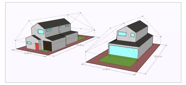
Figure 2 – Example of a 180m<sup>2</sup>, two-storey dwelling on flat, 300m<sup>2</sup> lot complying with all LDSRZ standards
