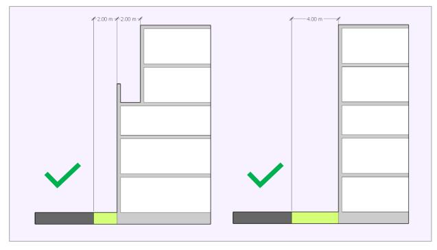
Figure 12 – Differing application of potential upper-storey setback within the HDRZ. The building on the right can utilise a greater front yard setback in lieu of the upper-storey setback.
