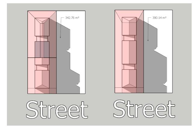
Figure 7 - Shading difference between Option 1 (right) and Option 2 (left). Model shot is taken at 3pm on 21 September with the models shown fully compliant with all standards.
