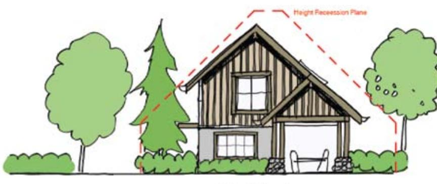
Using a gable roof design shapes the main form of the building and the smaller enclosed verandah. Overhanging eaves, verandah posts with stone base and a variety of materials provide visual interest while the simple form and use of low cost materials make this house fairly simple and affordable to construct.
