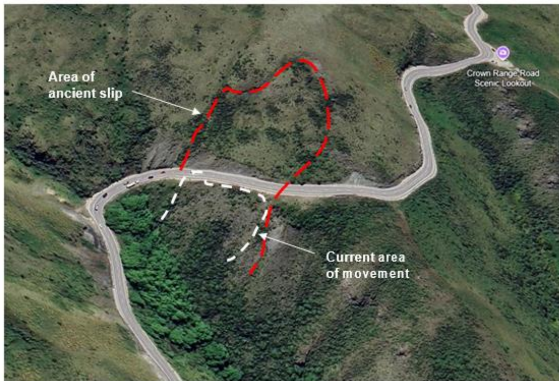
Figure 6. Inferred extent of potential slope instability at site 3 from Google Earth. Historic head scarp above the road is clearly visible.
