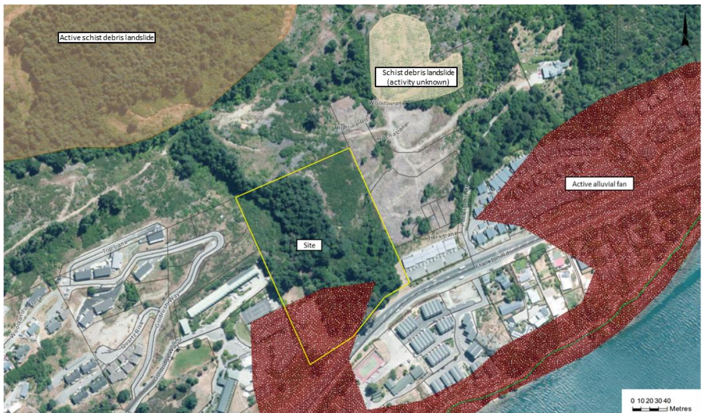
Figure 2: Site Boundary and Mapped Natural Hazards
