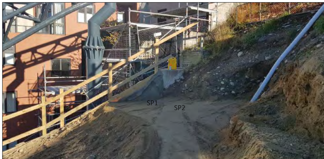
Photo 1: 1.5 m fill testing. Test locations indicated on the photo.
