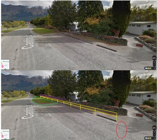
Cut back vegetation protruding through school fence (purple) to be achieved through volunteers Grass verge (green) to be scraped off and drainage sorted by local contractor sealed by council Traffic barrier (yellow) to be sourced and installed by council Small traffic island (red) sourced and installed by council East and West ends of Cantire repaired by council
