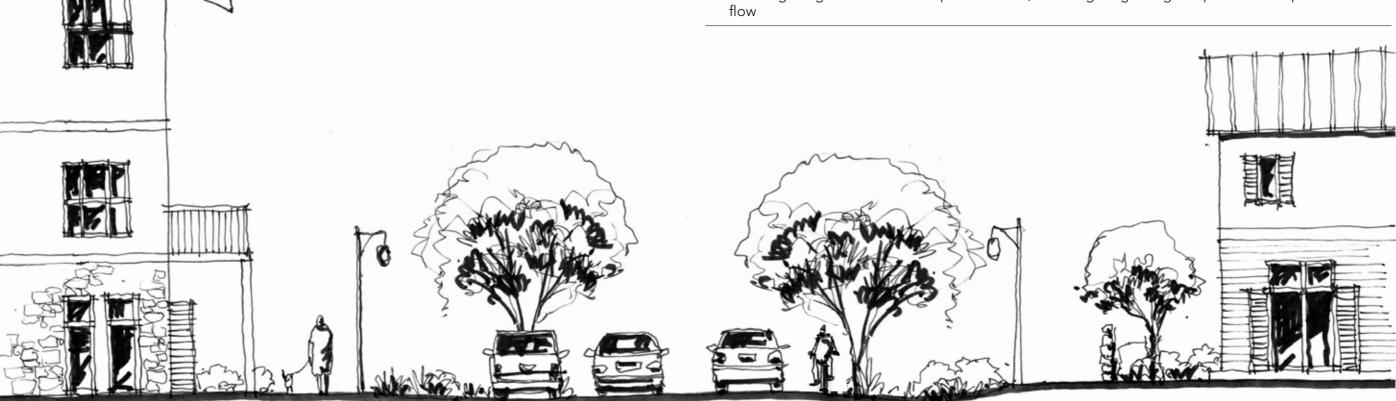
2.3m 1.8m 3m Footpath 3m Footpath 1.7m 1.7m Residential development 7m Carriageway Residential development Parking lane Cycle lane Landscaped Landscaped edge/ edge/ stormwater stormwater swale swale
