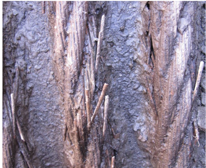
Figure 9. Example diagram and photo of brittle failure of the wires on the TL US location
