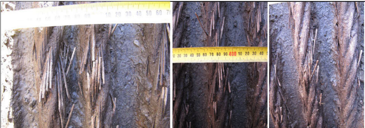
Figure 8. Cable damage on the True Left Upstream side
