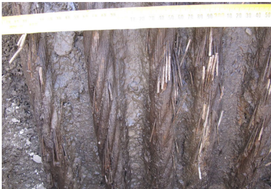
Figure 10. Damage to the two downstream most cables and the central three cables
