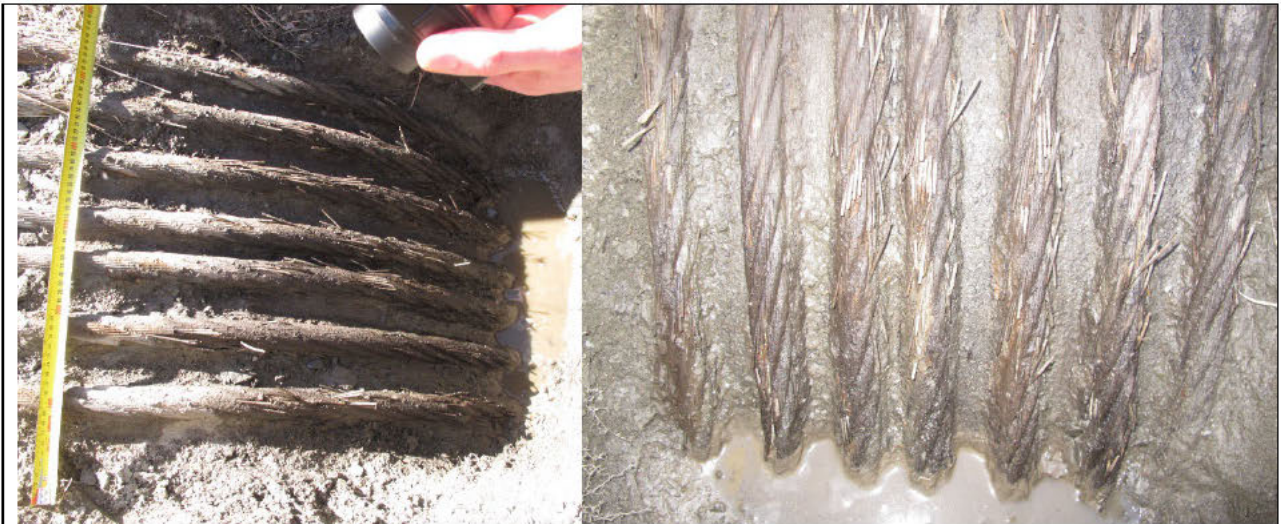
Figure 7 Cable Damage at rollover. Behind the cables is a radiused steel plate. The water visible was used to wash the cables
