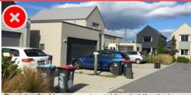
Provision for bins was not considered at the design stage or were located in an inconvenient location resulting in their placement in the front yard.
