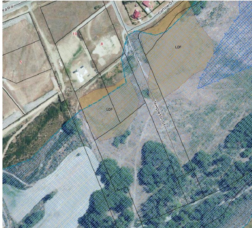
Figure 12: QLDC webmap image showing the flooding hazard on the site. The 'LDF' annotation represents a potential former landfill.
