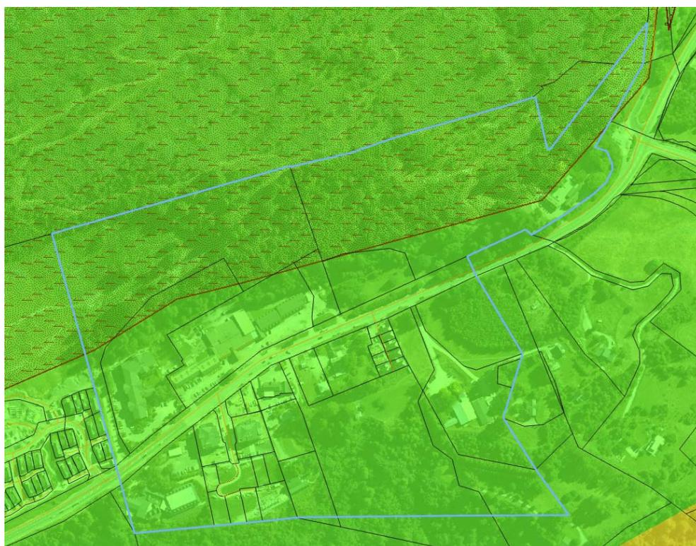
**Figure 7: Hazards Map for Arthurs Point North, outline shown with blue line. Green shows areas of nil to low risk liquefaction. Brown speckled overlay is Active Schist Debris Landslides hazard. Snip taken 19/02/2020.**
