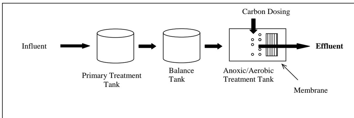
A MBR system is a combination of the activated sludge process (a wastewater treatment process characterised by a suspended growth of biomass) with a micro- or ultra-filtration system that rejects particles. MBRs have two basic configurations: (1) an integrated configuration that uses membranes immersed in the bioreactor (as above) and (2) a re-circulating configuration where the mixed liquor circulates through a membrane module situated outside the bioreactor.
