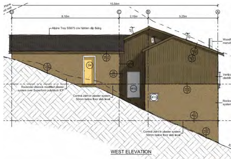
West Elevation facing subject lot -3 Conifer Lane
