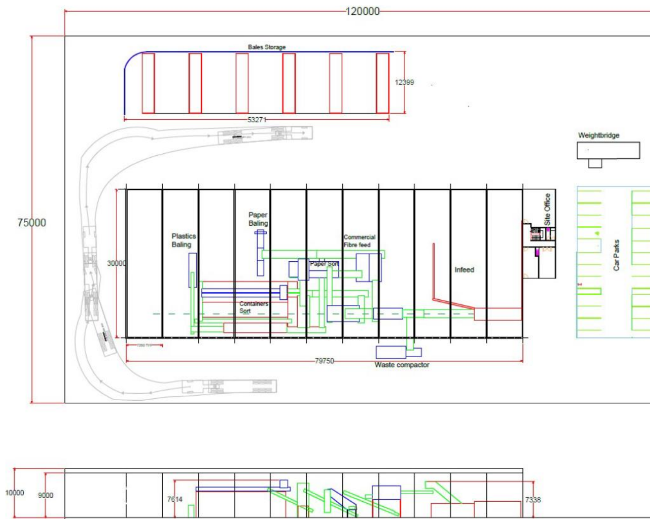
Figure 2 Concept layout for 5 tonne per hour MRF
