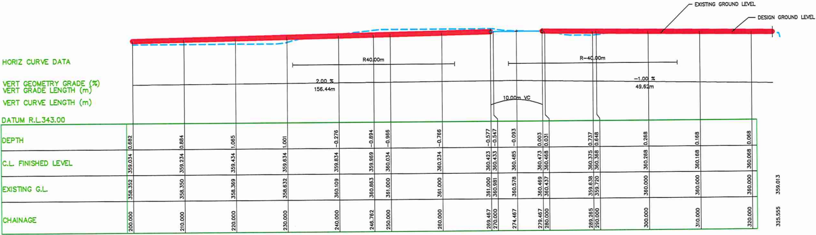
LONGSECTION - ACCESSWAY 002 A1 HORIZ SCALE 1 : 250 A1 VERT SCALE 1 : 250
