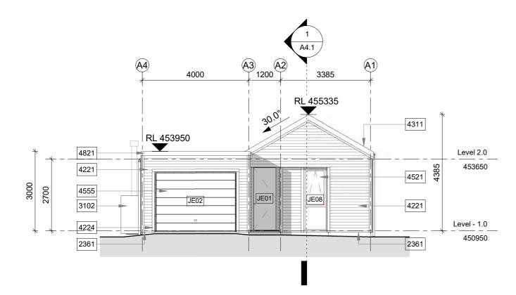
A) South Elevation 2 A2.1 Scale 1:100
