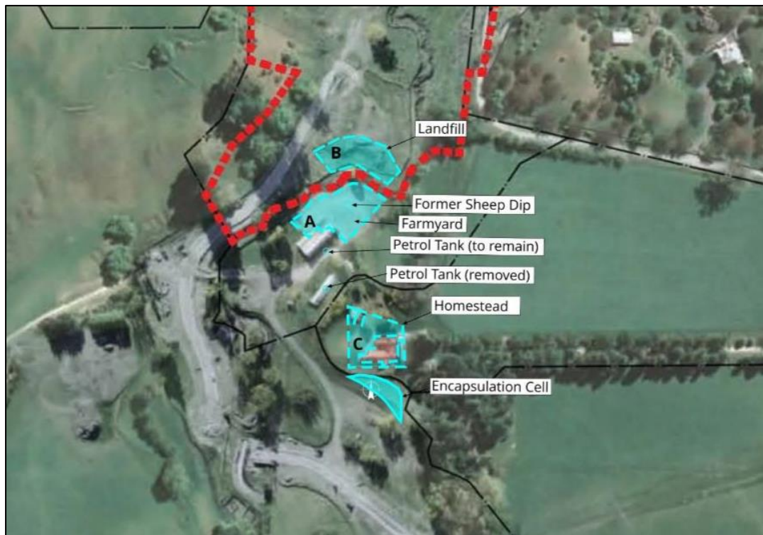
Figure 5: Showing three areas of remediated contamination (A, B and C) and the encapsulation cell
