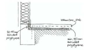
A method of insulating a slab edge
