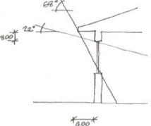
A glazed door with an eave 300mm above the head of the door needs an eave of about 800mm
