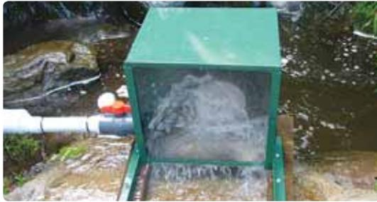
Close-up of a Pelton wheel impulse turbine. The water returns to the same catchment that it was diverted from.
