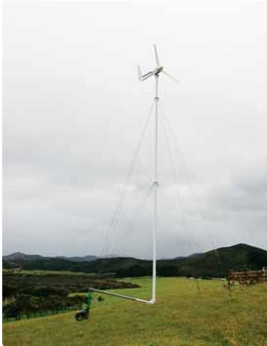
Pole mounted, with guy wires, three-bladed horizontal-axis micro wind turbine with a tilting mechanism.
