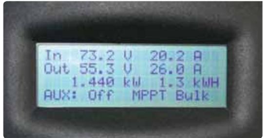
Example of a display unit on a grid-connected photovoltaic system.
