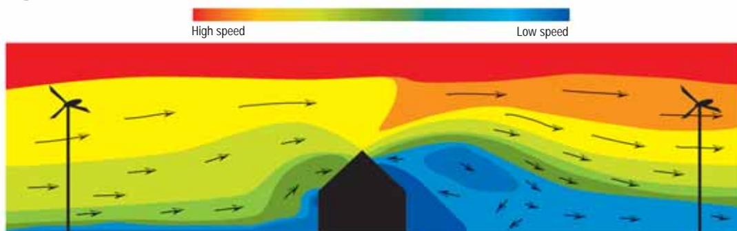
Pole-mounted turbines should be located away from obstructions such as building or trees. Taller poles or towers are required to position turbines in stronger and more consistent winds.
