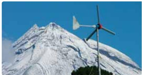
Pole-mounted, with guy wires, three-bladed horizontal-axis micro wind turbine.
