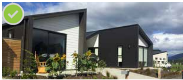
Buildings are broken down into clearly defineable units assisting legibility and reducing the perceived mass of buildings.
