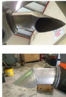
Photo B: Photo of secondary muffler attached to existing primary muffler. Reference / property of Hydro Attack©
