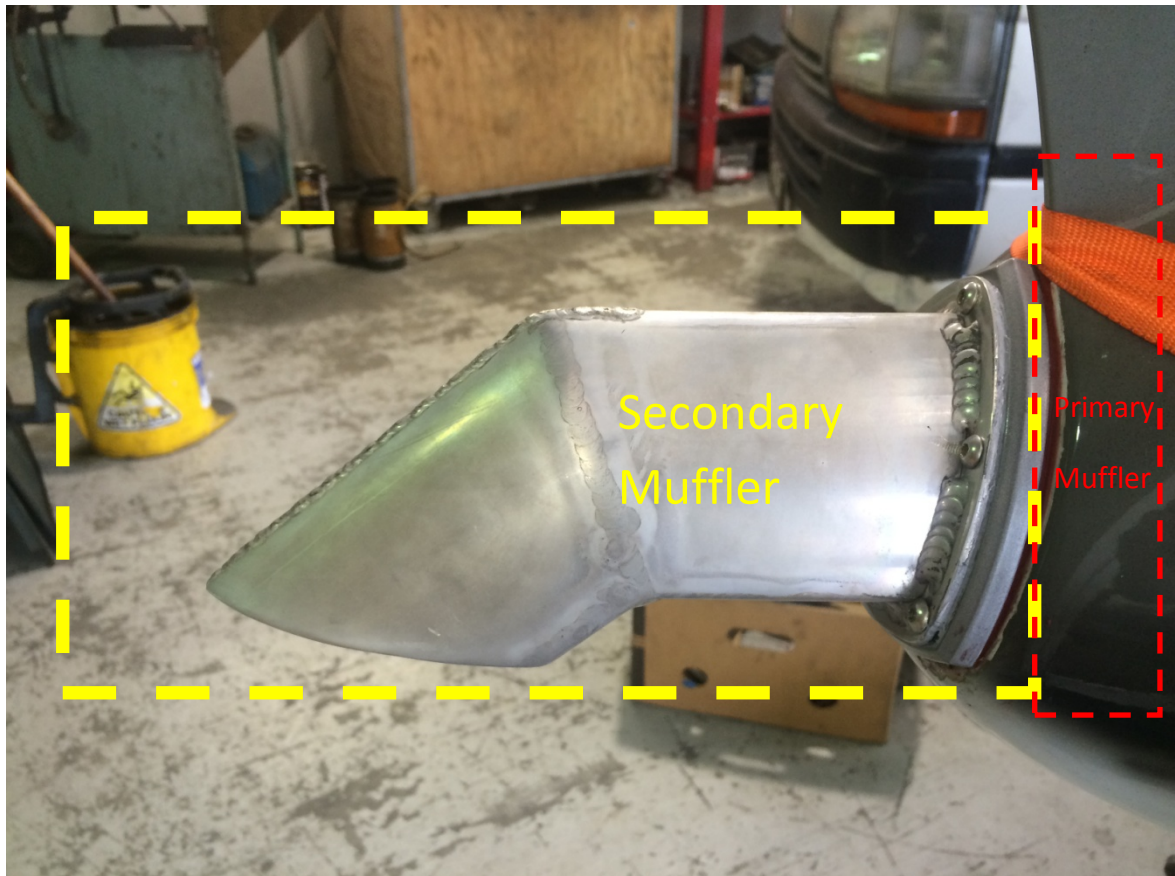
Photo C: Enlarged photo of secondary muffler attached to existing primary muffler. Reference / property of Hydro Attack©
