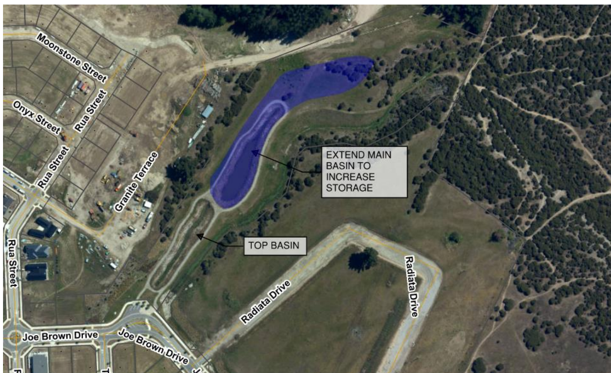
Figure 8-1 Sketch of proposed basin modifications. Pipework not shown. (Base map: QLDC GIS)
