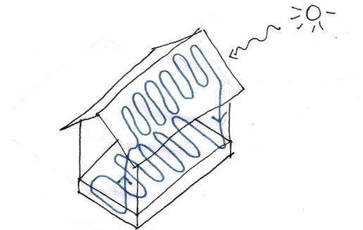
In-slab solar heating
