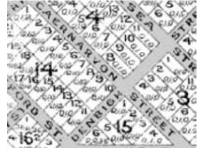
Rectangular lot pattern. The historic lot size and was 1 rood or 1/4 acre.
