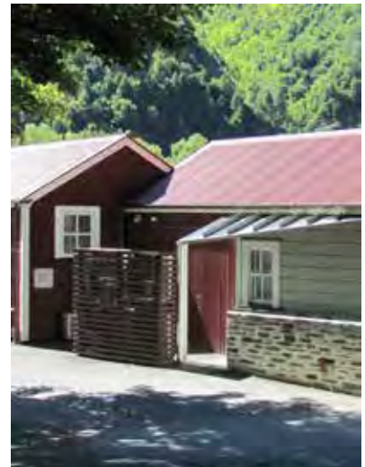
The same development viewed from Arrow Lane, reflecting traditional shed form, but retaining single storey elevation to Arrow Lane and promoting varied setbacks off the lane.
