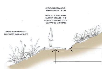
SMALL CHANNEL TO LINE INSIDE EDGE OF PATHWAY. PATHWAY TO SLOPE IN ONE DIRECTION TOWARDS THE CHANNEL
