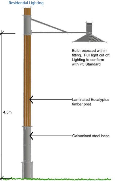
Selected downlight fitting. Light attachment to timber or steel and timber bollard
