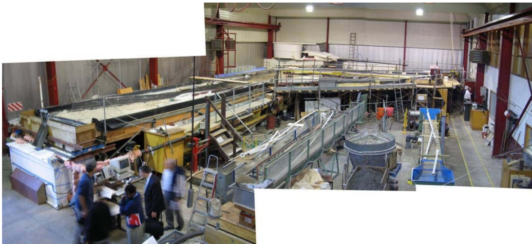
Figure 6.1: Physical model of Shotover River delta
